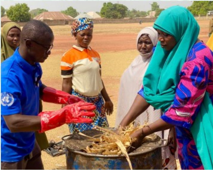
A training facilitator and women participants filling up maize husk into a carbonizer during a practical production of biomass briquettes in Kaduna state
